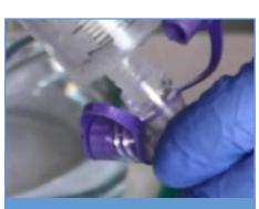
Connect syringe to the tube, being careful not to over-tighten
