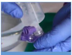
Connect syringe to the tube, being careful not to over-tighten
