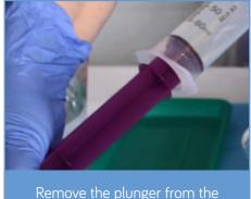
Remove the plunger from the syringe barrel
