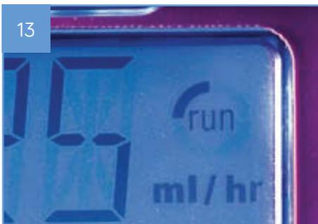
The RUN symbol will rotate to indicate that the pump is working
